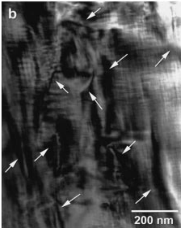
FIGURE 6. Irregular tweeds associated with deformation (a) (CT 15) Both directions of the tweed become coarser between two subgrain boundaries, without developing a single preferred direction. (b) (Vz 670) A highly deformed, irregular tweed. Arrows show dislocations.
