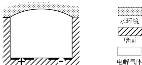
(c) 电解气泡覆盖微凹坑,阻隔反应 (c) Blocking reaction by covering the well with bubble
