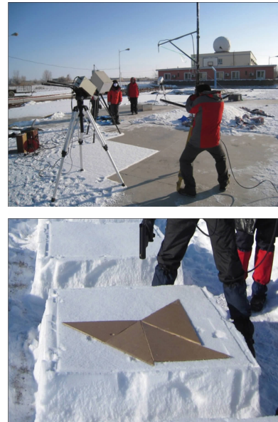
Fig. 2 The in situ measurement of spectral reflectance of different fractional snow cover
