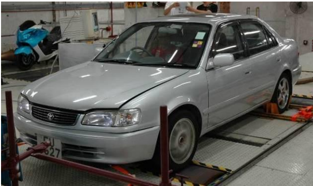
Fig. 7. Experiments on revolving drum test bench
