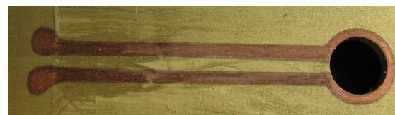
Fig. 9. Surface coating sensor after crack monitoring experiment
