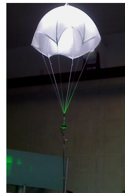
Fig. 11. Wind tunnel tests of parachute
