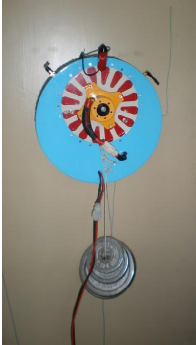
Fig. 13. BIT Climber at work with a load of 59 N
