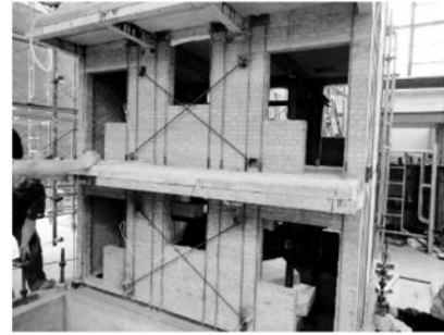
图4 模型二交叉斜撑布置(1,2层) Fig. 4 Cross bracing struts at first two stories of model-two
