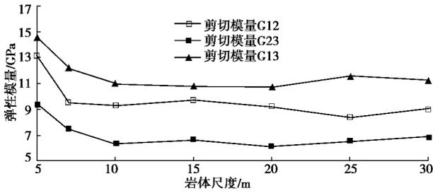
Fig. 6 Relationship between deformation parameters  $G_{12}$ ,  $G_{23}$ ,  $G_{13}$  and rock mass scale
