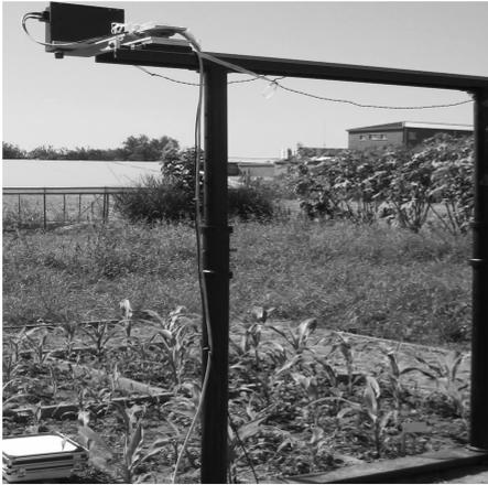
Fig. 1 Acquisition system of hyperspectral imaging
