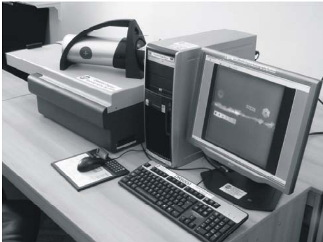
Fig. 2. Test stand equipped with a DR6000 system for digital radiography
