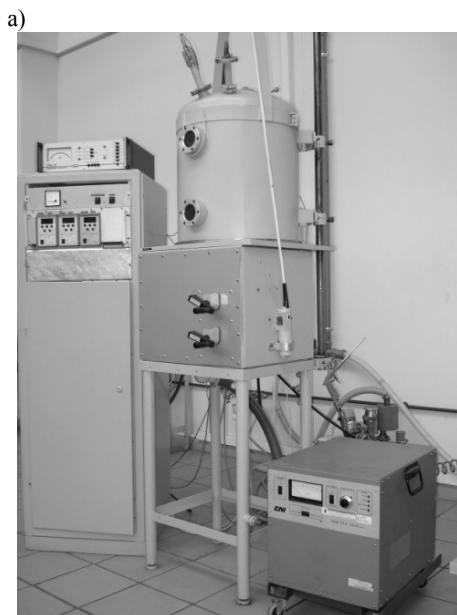
Fig. 2. General view (a) and scheme (b) of carbon coatings apparatus by RF PACVD method
