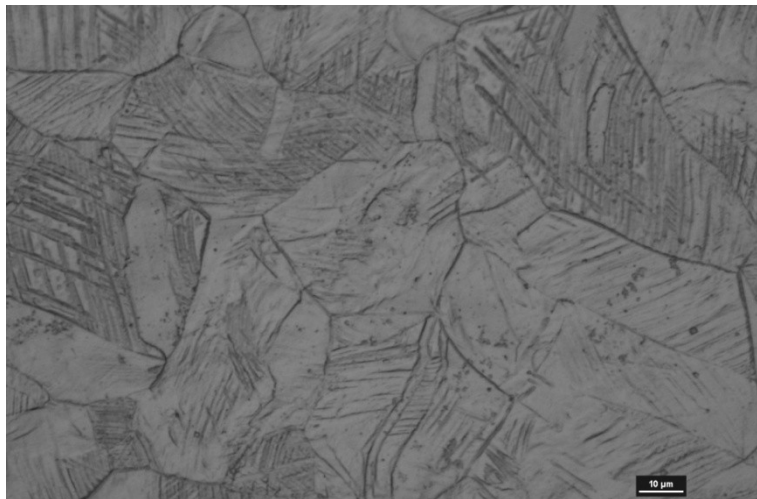
Fig. 1. AISI 316L microstructure after supersaturation (austenite with twins)
