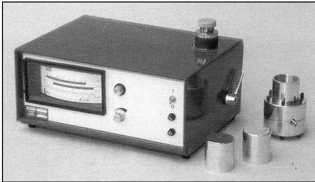
Fig. 1. Apparatus for determination of moulding sand permeability LPIR-1 [5]
