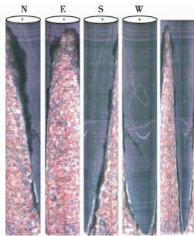
图1 钻孔ZK3中基性岩脉与花岗岩的接触关系 Fig. 1 Contact between basic dykes and granite in ZK3
