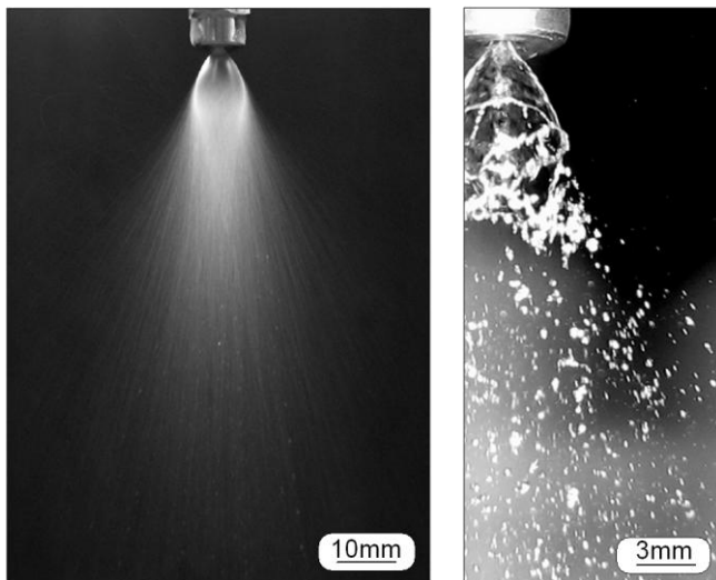
Fig. 3. Stream of sprayed water with use of designed rotary sprayer
