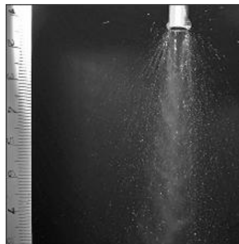
Fig. 6. Stream of water mist under pressure 0.3/0.38 MPa cooling the die surface
