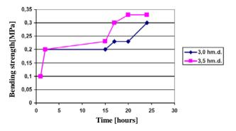
Fig. 4. Dependence of result fortress at curve ex tempore filling mixtures of various resin concentration of opening material Chromit- JAP Třinec
