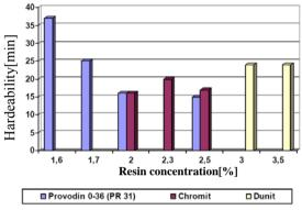
Fig. 2. Influence of resin concentration at hardeability of mixtures for different types of opening materials
