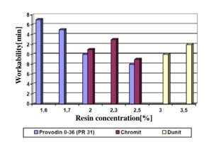
Fig. 1. Influence of resin concentration at workability of mixtures for different types of opening materials
