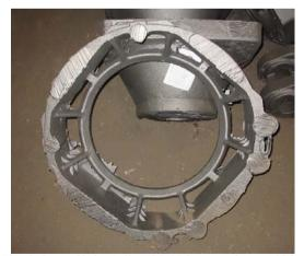
Fig. 6. Cast "Skriňa" alloy GS 45.3. gross charge 102 kg
