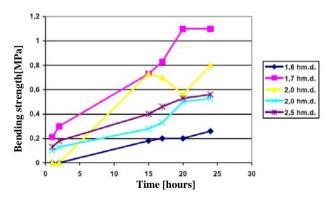
Fig. 3. Dependence of result fortress at curve ex tempore filling mixtures of various resin concentration of opening material Provodin PR 31
