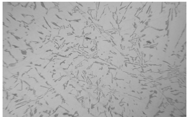
Fig. 3. Microstructure of Al-Si alloy influenced by direct electrical current of 15 A, 100x ext, etched with 0,5% HF
