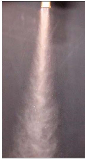
Fig. 4. Stream of water mist cooling the die surface
