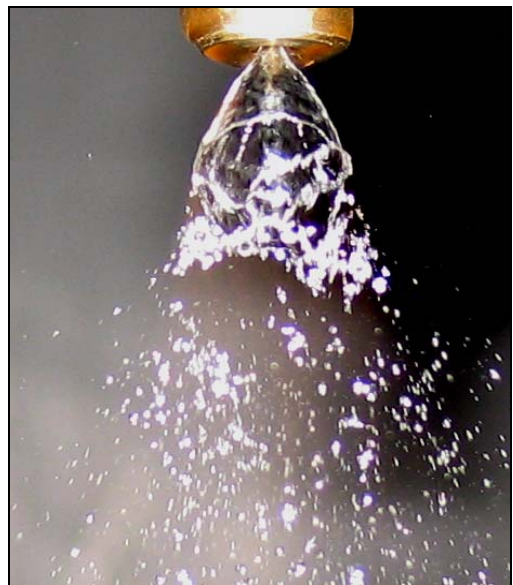
Fig. 3. Streams of sprayed water with use of designed rotary sprayer, magnification 3 times
