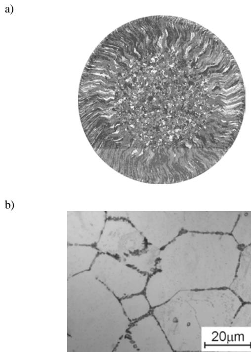
Fig. 4. Macro- (a) and microstructure (b) of aluminium EN AW-Al99,5 after casting with influence of IRPM
