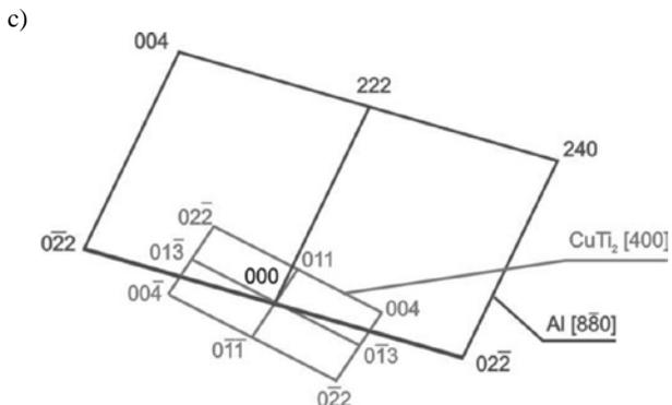
Fig. 9. a): Structure of thin foil from aluminium EN AW-A199,5 after inoculation with (Ti + B) – 30000x , b): diffraction pattern from the area as in fig. a, c): solution of the diffraction pattern from fig. b
