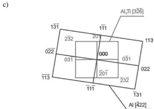
Fig. 8. a): Structure of thin foil from aluminium EN AW-Al99,5 after inoculation with (Ti + B) – 30000x , b): diffraction pattern from the area as in fig. a, c): solution of the diffraction pattern from fig. b
