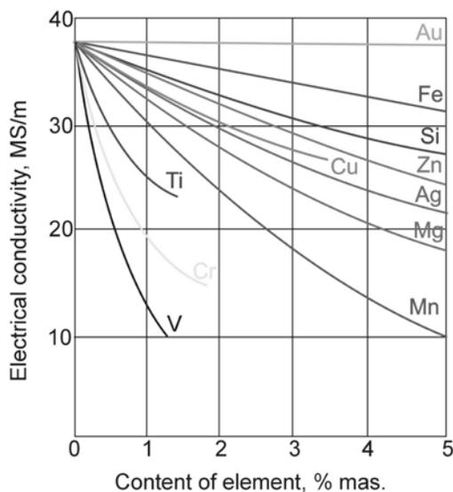
Fig. 1. Influence of different elements on electrical conductivity of EN AW-Al99,99 [9]
