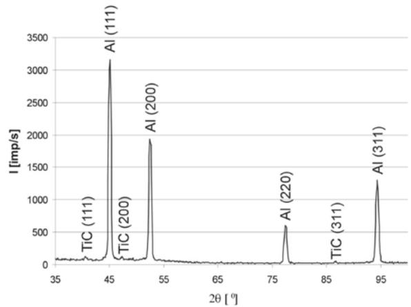
Fig. 7. X-ray diffraction of aluminium EN AW-Al 99,5 after inoculations Ti and B
