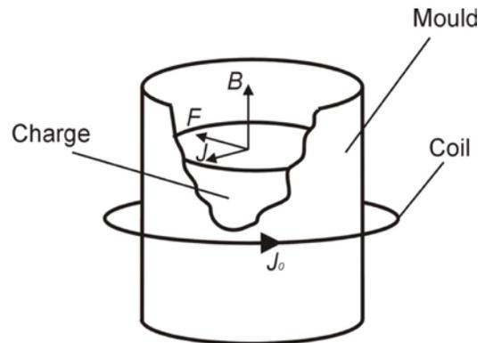
Fig. 2. Generation of liquide metal movement in mould [10]
