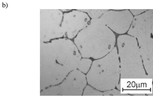
Fig. 6. Macro- (a) and microstructure (b) of aluminium EN AW-Al99,5 which was casted with influence of IRPM and with inoculation with 25ppm Ti + 5ppm B
