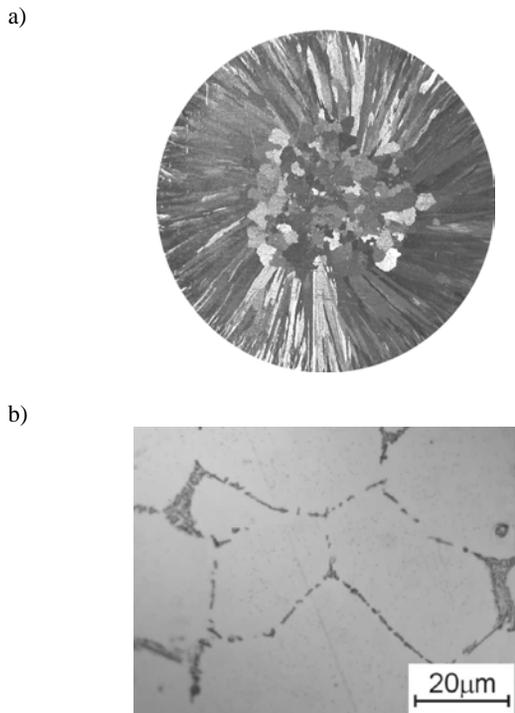
Fig. 3. Macro- (a) and microstructure (b) of aluminium EN AW-Al99,5 without inoculation
