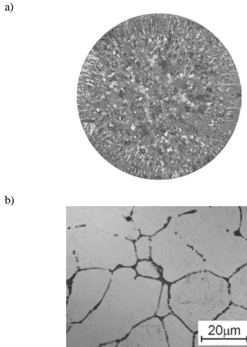
Fig. 5. Macro- (a) and microstructure (b) of aluminium EN AW-Al99,5 after inoculation with 25ppm Ti + 5ppm B
