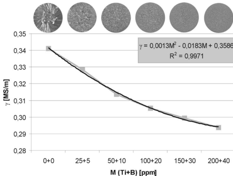
Fig. 10. Electrical conductivity (γ) of aluminum EN AW-A199,5 in quantity of inoculants M (Ti + B) function
