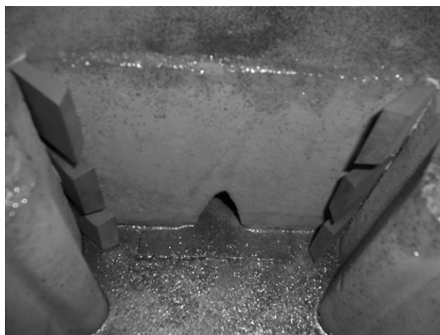
Fig. 3. View of mould cavity with reinforcement plates in corners
