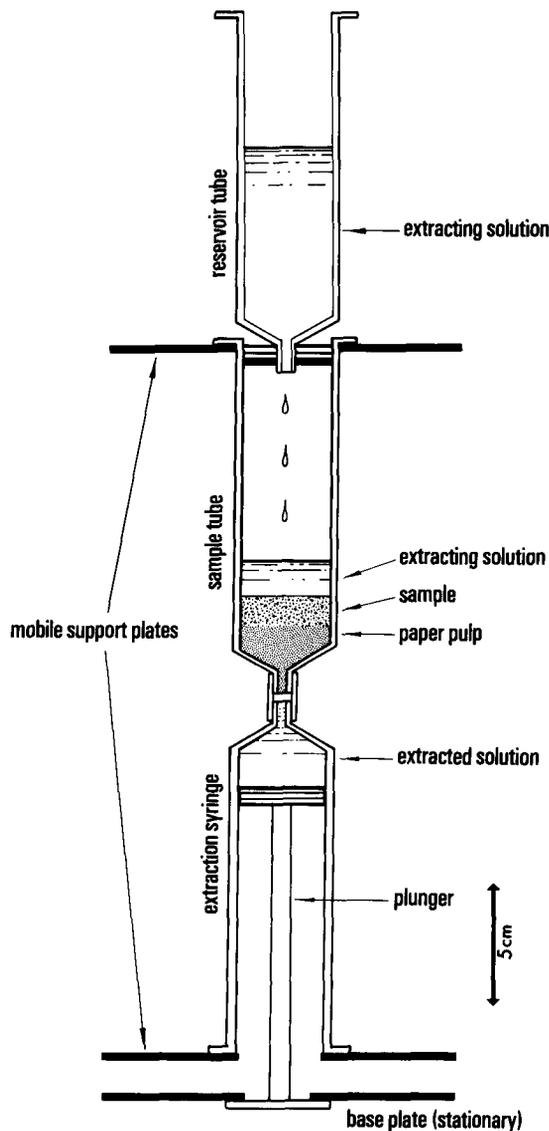
Figure 1. Cross section of extraction assembly, mechanical extractor.
