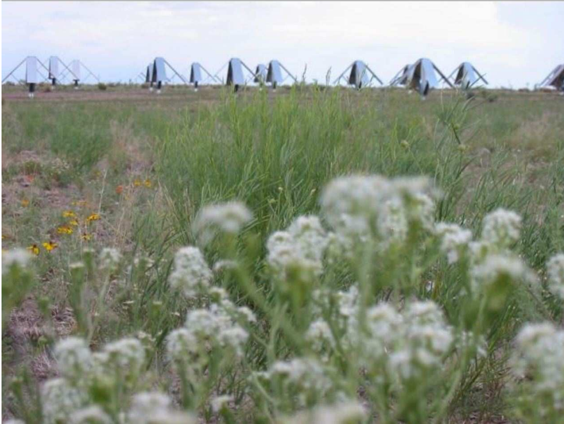
Fig. 1.— Photo of the Long Wavelength Demonstrator Array in New Mexico showing the individual dual-polarization stands. Each stand consists of four droopy blades which provide dual-polarization capabilities.
