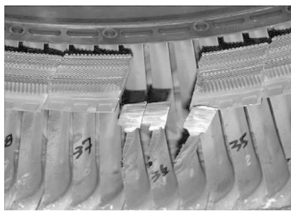
图1 第36组LPT4静子叶片叶尖翘起及摩擦痕迹 Fig. 1 Abrasion mark and cocked appearance of No. 36 LPT4 vanes
