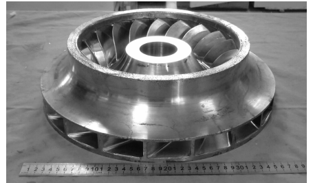
图5 电火花精加工完成后的三元流闭式叶轮 Fig. 5 3D-flow closed impeller after completion of precision work by NC-EDM
