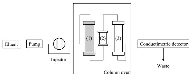
Fig. 4 Schematic diagram of urea determination by an immobilized urease column on-line to the IC system. (1) Immobilized urease column, (2) guard column, (3) YK-421 column.
