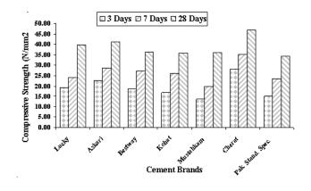
Figure 1: Compressive strength of different brands of cements
