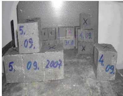
Fig. 1. – Samples of polymer concrete
