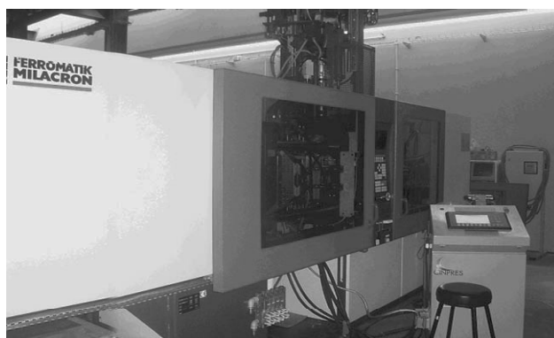
Fig. 1. Injection molding machine with special mold , remotely operated
