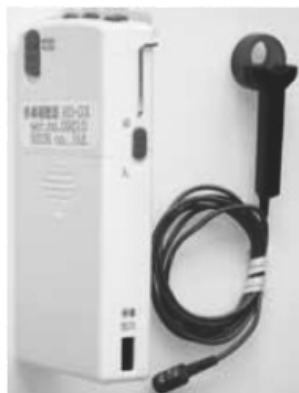
Fig. 11. Cartilage conduction hearing aid developed in this study. It consists of a cartilage transducer (right) and microphone/amplifier complex (white box on left). The red circle is convenient to fix the cartilage conduction transducer to the tragus
