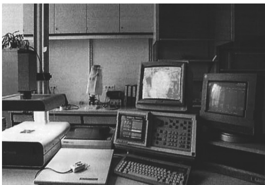
Fig. 7. Equipment for measuring the pesticide coverage on WSP with Optomax Image Analysis system
