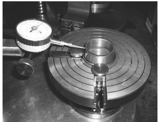
Fig. 4. Photography of measure of run-out of main bearing way to the broad end face
