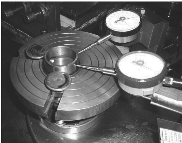
Fig. 3. Photography of measure of ovality and lobing parameters
