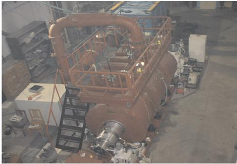
Fig. 1 Photo of pulsed X-ray source based on IVA/RPD
