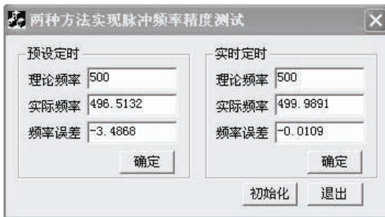
图 5 两种方法实现脉冲频率精度测试 Fig.5 Test for pulse frequency precision of the two realization methods
