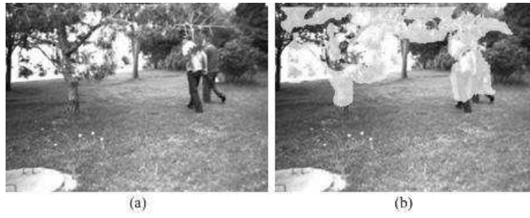
Fig. 9 The positive obstacles (tree, bushes and moving persons) and their detection results (the obstacles are indicated by light blue)
