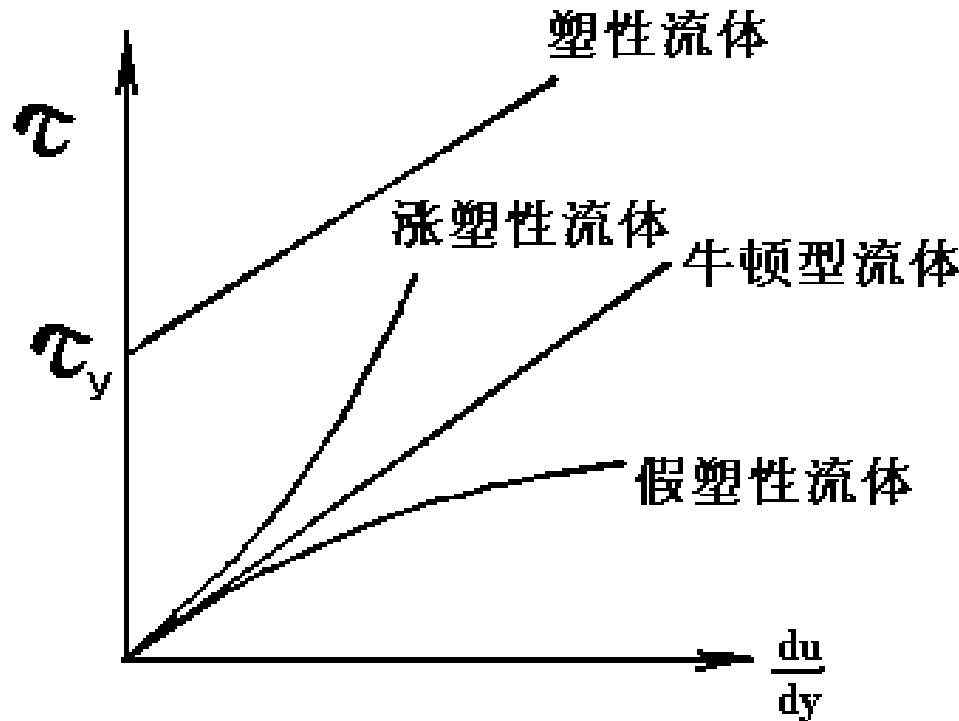
$$\text{粘度 } \mu = \frac{\tau}{du/dy} = f\left(\frac{du}{dy}\right)$$
