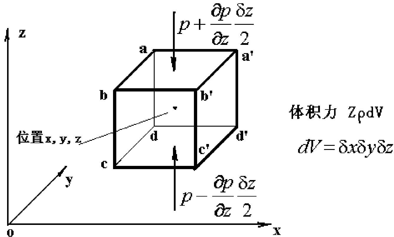
$$Z\rho dV + \left[ \left( p + \frac{\partial p}{\partial z} \frac{\delta z}{2} \right) - \left( p - \frac{\partial p}{\partial z} \frac{\delta z}{2} \right) \right] \delta x \delta y = 0$$
