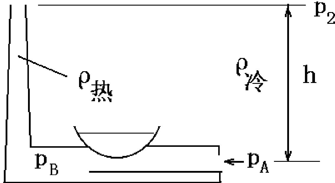
$$p_A = p_2 + \rho_{\text{冷}} gh \quad \text{由于 } \rho_{\text{冷}} > \rho_{\text{热}}$$
