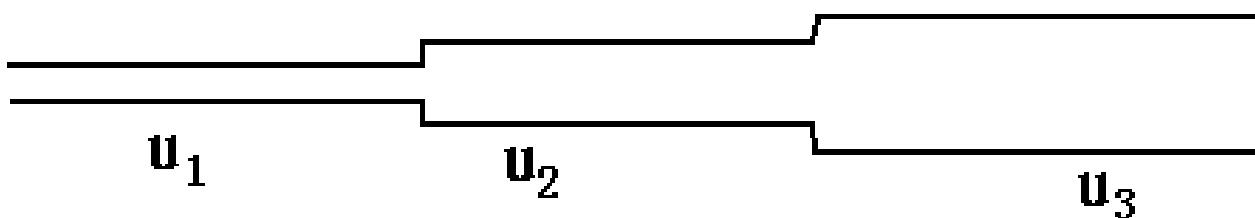
方程特点:  $h_{f\text{总}} = h_{f1} + h_{f2} + h_{f3}$
