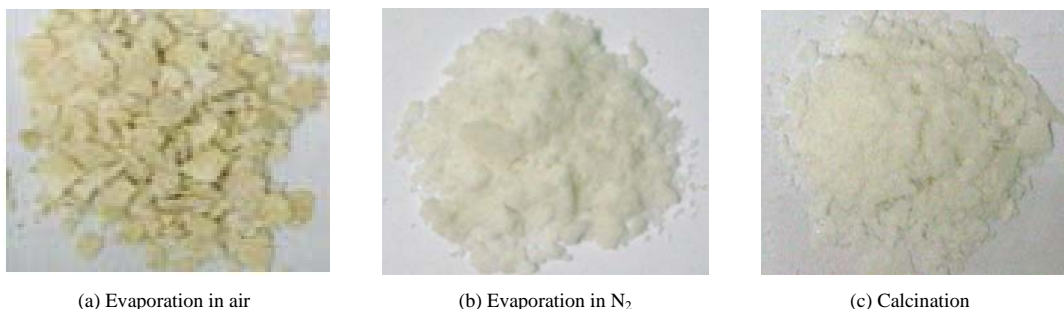
图 8 不同条件下蒸发所得硫酸钠粉末 Fig.8 Sodium sulfate powder products obtained by evaporation at different conditions
