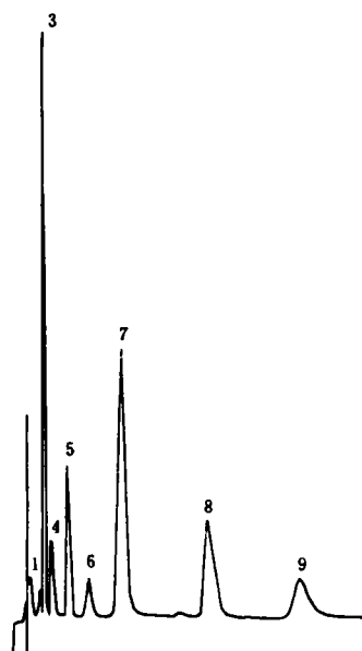
Fig 1 HPLC chromatogram of catechins, alkaloids and internal standard. 1. Theobromine (Tb); 2. Theophylline (Tp); 3. Caffeine (Caf); 4. (-)-Eicatechin gallate (EGC); 5. (+)-Catechin (C); 6. (-)-Epicatechin (EC); 7. (-)-Epigallocatechin gallate (EGCG); 8. (-)-Epigallocatechin (ECG); 9. Diclofenamide (DCF).
