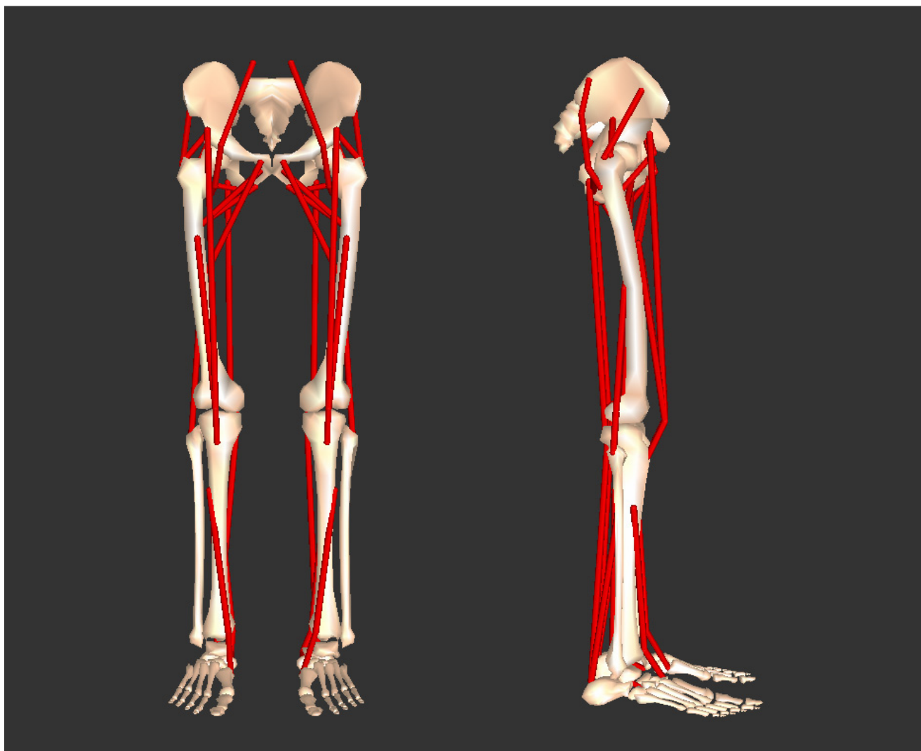
Figure 1 The musculoskeletal model developed for this study. The simulation model contained 9 rigid body segments, and the degrees of freedom of the model was 20.
