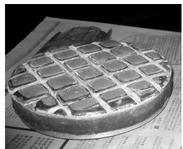
Fig. 7 150 mm passive semi-rigid lap
