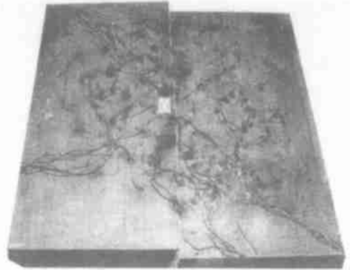
图 5 Big5 模型有阻力摩擦滑动裂隙错动照片 Fig. 5 Photo of crack dislocation of model Big5 during resistive frictional slipping
