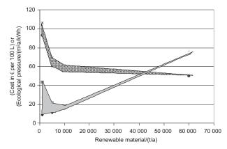
**Fig. 1.** Ecology of scale *vs.* economy of scale:  $\square$  ecological pressure of the options according to the SPI method in m<sup>2</sup>a/kWh heating value of ethanol,  $\boxtimes$  costs in  $\pounds$  of 100 L of ethanol for the alternatives
