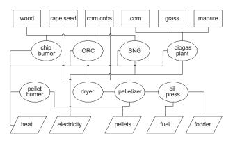
**Fig. 2.** Maximum structure of a regional multifunctional centre utilising wood, corn, grass, oil seed and straw; ORC – organic Rankine cycle, SNG – synthetic natural gas production
