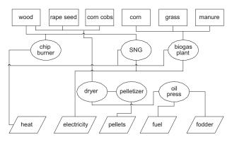
Fig. 3. Optimum structure of the given case study
