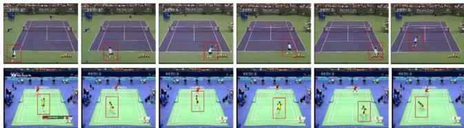
Fig. 4. Results of player tracking and stabilization, the rectangle region represents the stabilized human-centric figure.
