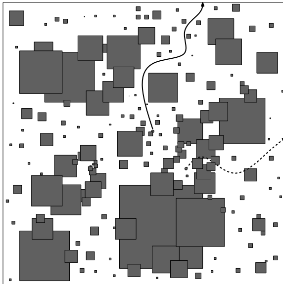
Figure 1: Sketch of a Poisson square soup. The point at the end of the solid line can be connected to the boundary by a path that does not cross the soup, and thus belongs to the carpet. The point at the end of the dotted line is completely surrounded by the soup and thus is not in the carpet.
