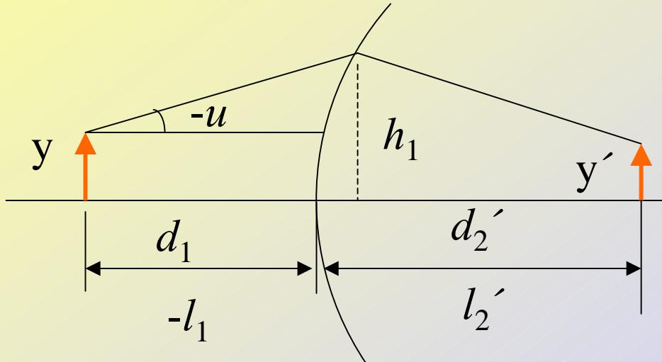
$$\therefore \begin{bmatrix} n_2' u_2' \\ y' \end{bmatrix}_B = B' \begin{bmatrix} 1 & 0 \\ -\frac{l_2'}{n_2'} & 1 \end{bmatrix} \begin{bmatrix} n_2' u_2' \\ h_2' \end{bmatrix}$$
