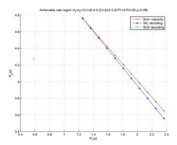
Fig. 3. SIC decoding, space PA. The achievable rate region at the NE versus the distribution of the coordination signal  $p \in [0, 1]$  for  $n_r = n_t = 10$ , r = [0.4, 0.2], t = [0.6, 0.3],  $\rho = 3dB$ ,  $P_1 = 5$ ,  $P_2 = 50$ . Varying p allows to move along a segment close to the sum-capacity, similar to SISO MAC.
