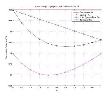
Fig. 2. SIC decoding, comparaison between the joint space-time PA and the two special cases: the space PA and temporal PA. Sum-rate efficiency versus the distribution of the coordination signal  $p \in [0,1]$  for  $n_r = n_t = 10$ , r = [0.3,0], t = [0.5,0.2],  $\rho = 4dB$ ,  $P_1 = 5$ ,  $P_2 = 50$ . The spatial PA outperforms the joint space-time PA (Braess paradox).
