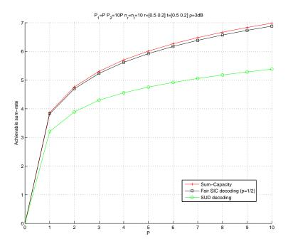
Fig. 1. Fair SIC (joint space-time power allocation) vs. SUD decoding. Achievable network sum-rate versus the available transmit power P for  $p = \frac{1}{2}$ ,  $n_r = n_t = 10$ , r = [0.5, 0.2], t = [0.5, 0.2],  $\rho = 3dB$ . The fair SIC performs much closer to the sum-capacity upper bound than SUD.
