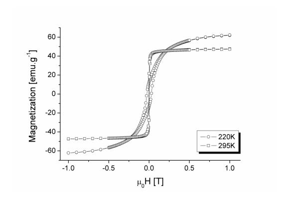
Temperature dependence of the magnetization for selected values of the in-plane applied magnetic field. The measurements were performed on cooling.
