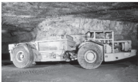
Fig 1. Traditional haulage truck with a combustion engine during work
