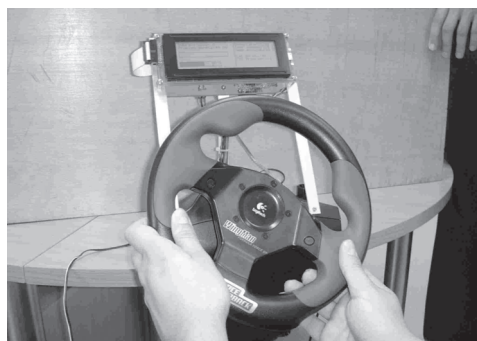
Fig 8. Wheel with ForceFeedback system with digital display
