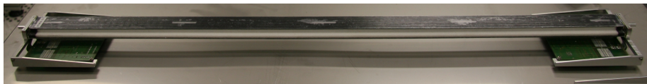
Figure 19: Photograph of a completed narrow module used in the testbeam. Two boards carrying front-end electronics are visible at the sides.
