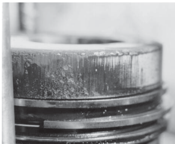
Fig. 1. The underneath of the piston surface after 200 motor-hours of exploitation using pure biodiesel (Liubarskis et al. 2002)
