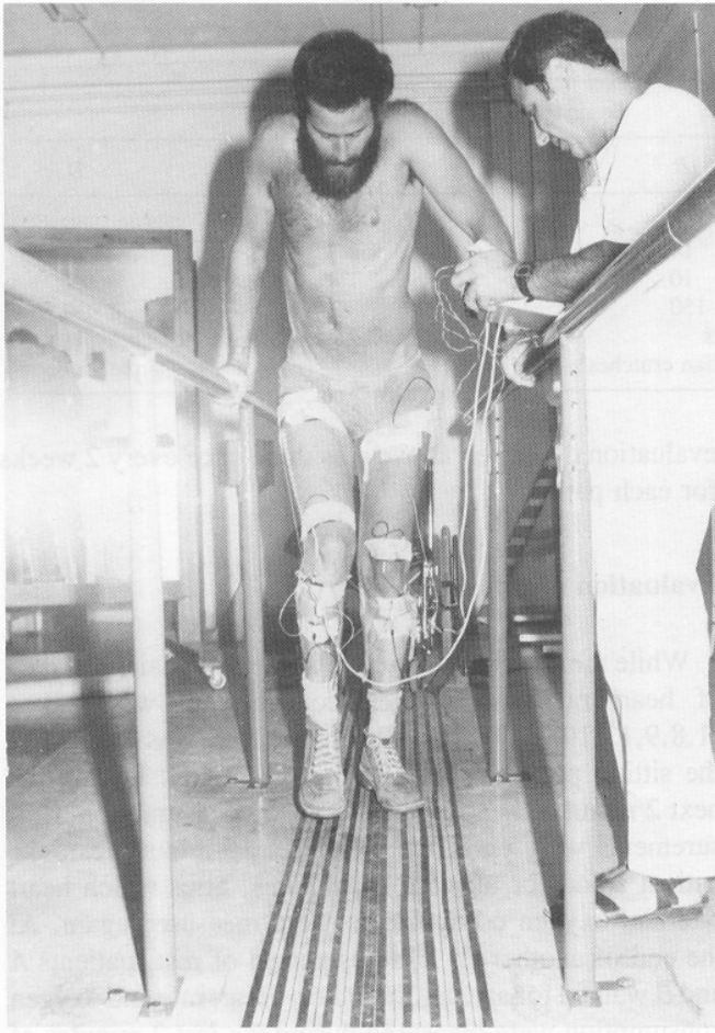
Figure 2 Patient B demonstrating flexion reflex during walking between parallel bars on the electric contact system and by which the time-distance parameters of the stride are monitored.
